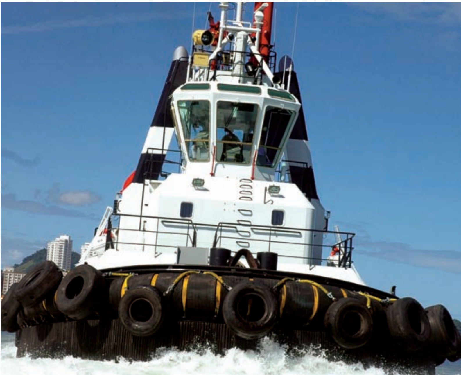
Above: The 72 ton bollard pull tug Aquarius. The Aquarius is an Azimuth Stern Drive (ASD) tug boat and was completed at our shipyard in Guaruja in 2006.
