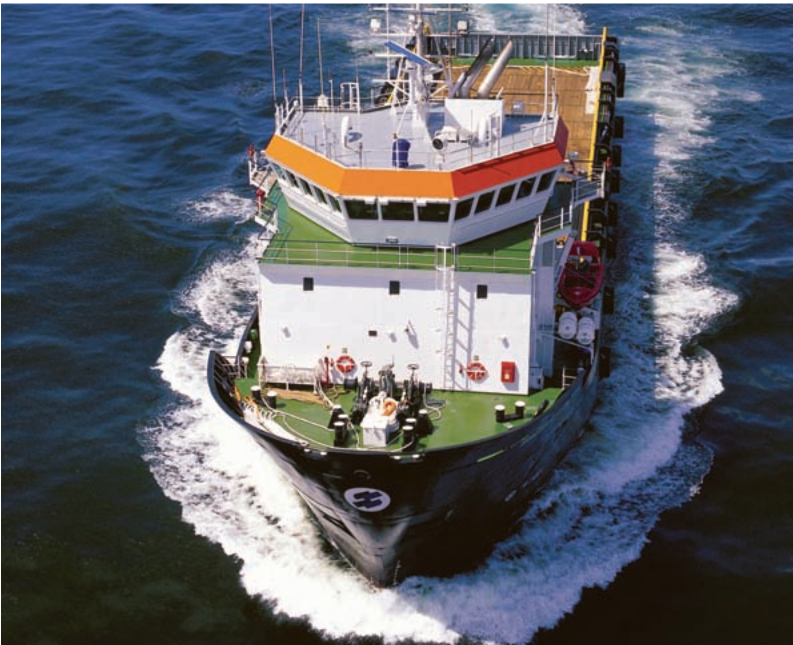
Above: the platform supply vessel Saveiros Albatroz. She is UT 755L designed by Rolls Royce Marine and has a length of 71,90 metres and breadth of 16 metres and operates along the Brazilian coastline.
